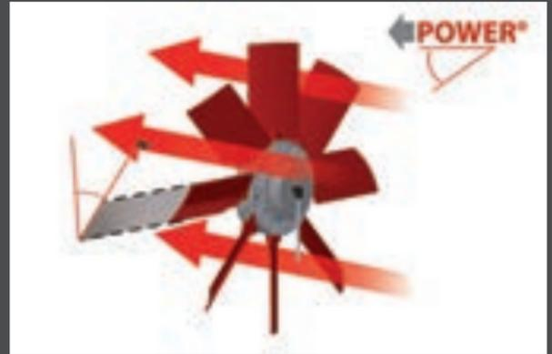
The power consumption of a fan depends on the angle of its blades. As CLEANFIX VP automatically adjusts its blades depending on the cooling requirements, it also automatically adjusts its power consumption. By using a low blade angle, savings of up to 60% in horse power consumption is possible.
