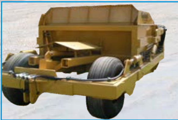
Safety shield protects ejector cylinders, rails, and guide rollers.
