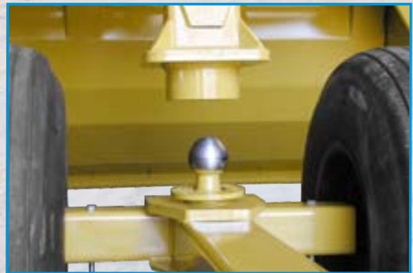
Large machined 4" ball for strength and smooth swivel of dolly.
