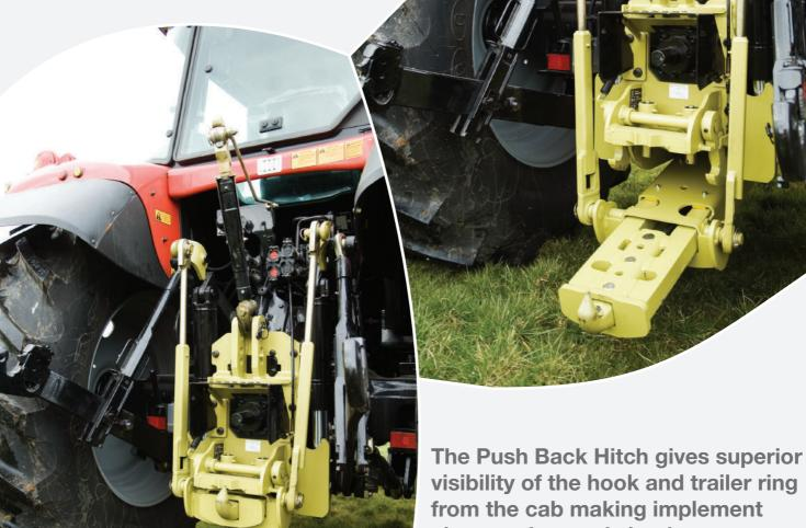
visibility of the hook and trailer ring from the cab making implement changes fast and simple.
